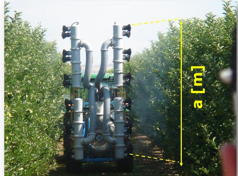
$$\text{Volumen [l/ha]} = \frac{\text{Caudal [l/min]} \times 600}{\mathbf{a} \text{ [m]} \times \text{Velocidad [km/h]}}$$
