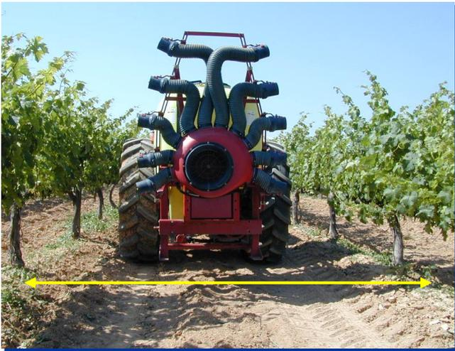
$$\frac{6 \text{ l/min}}{10 \text{ boquillas}} = 0.6 \text{ l/min}$$
