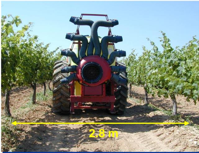
$$\frac{20.5 \text{ l/min}}{8 \text{ boquillas}} = 2.56 \text{ l/min}$$
