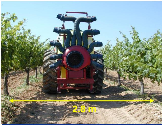
$$\frac{6.4 \text{ l/min}}{8 \text{ boquillas}} = 0.80 \text{ l/min}$$
