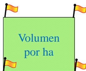
$$\frac{\text{Caudal } 1.6 \text{ L/min} \times \text{Factor } 600 \times \text{N}^\circ \text{ boquillas } 28}{\text{Barra } 14 \text{ m} \times \text{Velocidad } 5 \text{ km/h}} = 384 \text{ L/ha}$$
